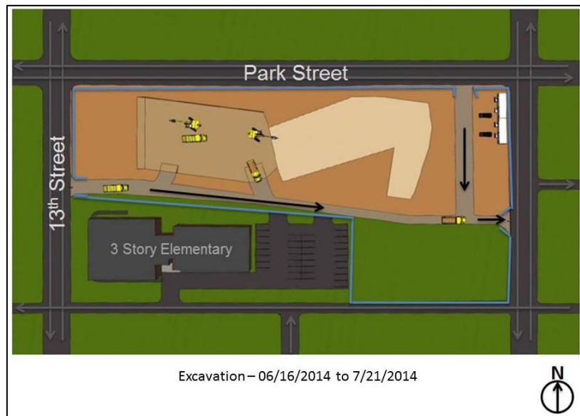
Figure 4: Excavation Site Plan
